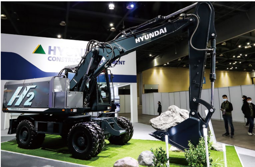
Hydrogen-powered excavator showcased at 2021 Construction Equipment Exhibition
