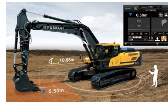
An example of using the Hi ASSIST technology for real-time surveying and automatic control
